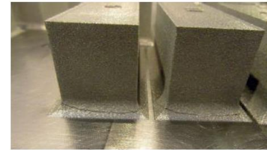
b) Cracks on the support interface
