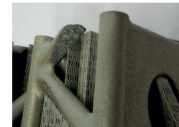
a) Colouring appearing in the downskin area
